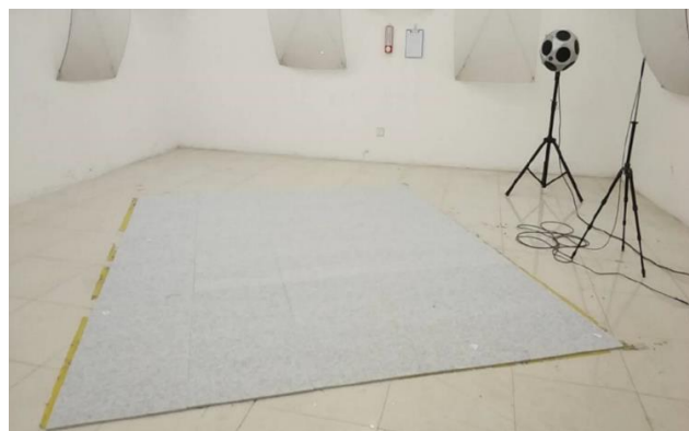
Test Setup: ISO 354:2003 and ISO 11654:1997
